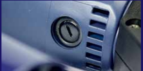
Fast and easily changeable carbon brush
