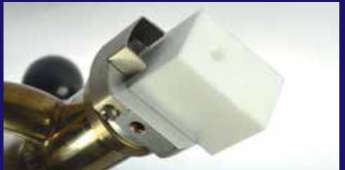
Quickly replaceable welding shoes result in high productivity
