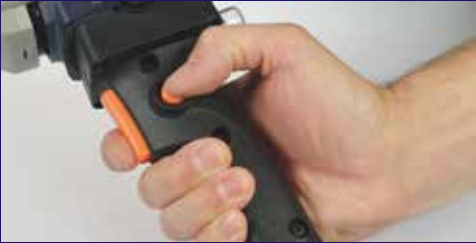
Locking button for continuous extrusion welding with little effort
